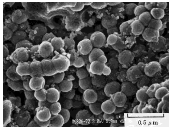
Figure 13 SEM micrograph of the etched surface of epoxy resin modified with acrylic rubber particles.
