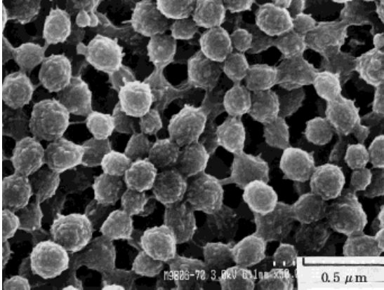
Figure 12 SEM micrograph of the etched surface of epoxy resin modified with core/shell acrylic particles.
